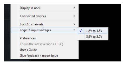
The lower voltage settings should work in most circumstances. The 5V setting is provided to reduce the likelihood of channel to channel crosstalk when using 5V signals. Crosstalk is developed, at least in part, by Logic16's long lead wires, fast rise/fall times, and is greatest when using 5V signals. Logic16's front end filters noise like this, but only up to a point. You should be able to have 8 different signals simultaneously switch without seeing crosstalk on adjacent signals.
